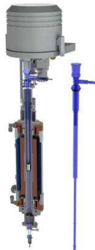
Figure 3 Cross section of the silica tube arrangement
