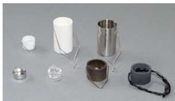
Figure 1 The TG mode with suspensions and crucibles
