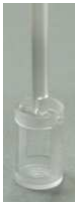
Figure 4: Picture of the sapphire attachment (crucible+suspension)
