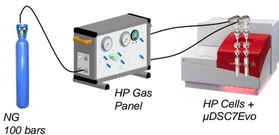
Figure 1 – Set-up for high pressure DSC tests
