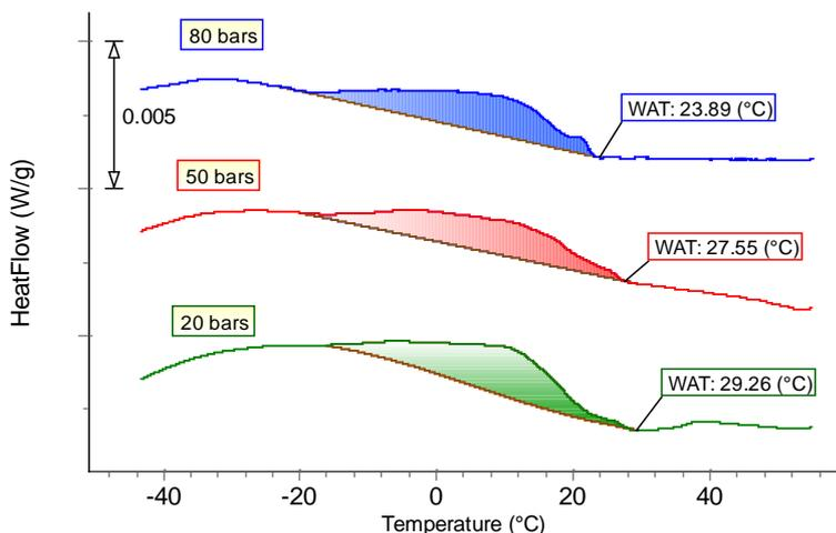
Figure 2 – Exothermic effects of wax precipitation
