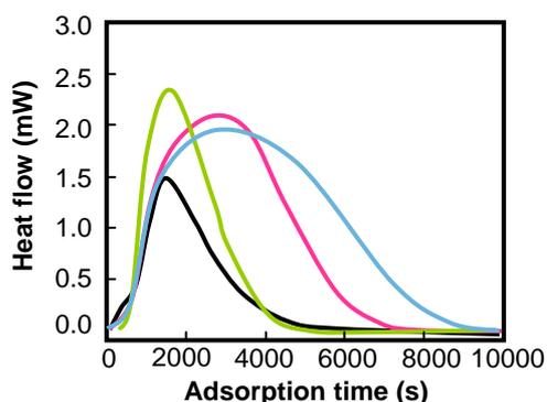
Heat of adsorption of sulfur compounds in hexadecane on NaY at 30 °C. All solutions contain 1800 ppm S except 4,6-DMDBT containing 900 ppm S :
