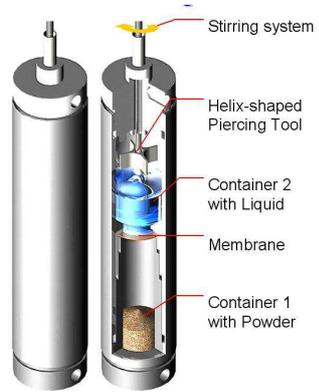
Figure 1 – Membrane mixing cell
