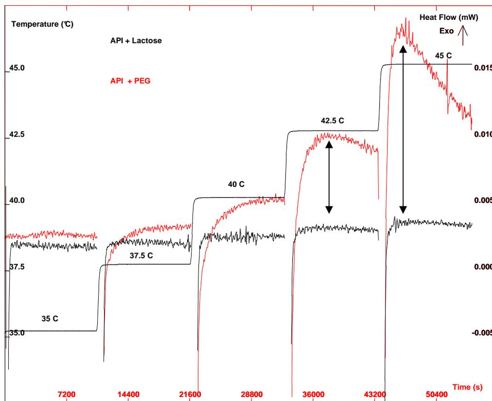
**Figure 1 – Comparison of the heat release of two formulation of the same API at different temperatures. The arrows point out the increase of heat production from the sample containing PEG**
