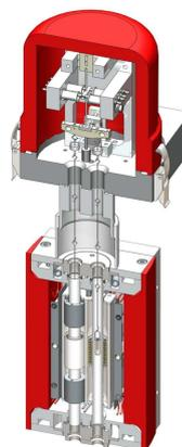
Figure 5 – Sensys TG-DSC cross-section
