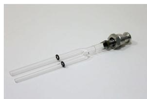
Figure 4 – Silica glass finger and the adaptation to Sensys DSC
