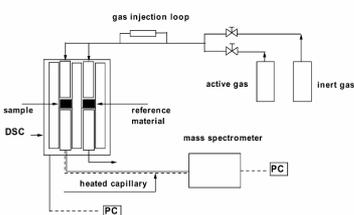
Figure 2 – Schematic representation of the Calvet type DSC with the injection loop and the MS coupling
