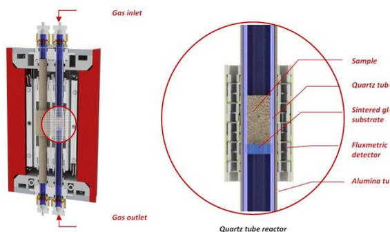
Figure 1 – Calvet type DSC cross section in the vertical mode with the quartz tube reactor
