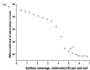
Figure 3 – Differential heats of adsorption of CO on CuY as a function of surface coverage
